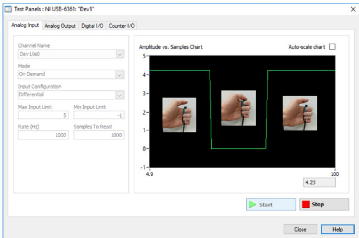
*Figure 2.* Graphical output measured in the NI Test Panel. We show that when the pickle switch is not activated (trigger button not pressed) a constant ~4.2 V is measured, and 0 V is measured when activated (trigger button pressed).
