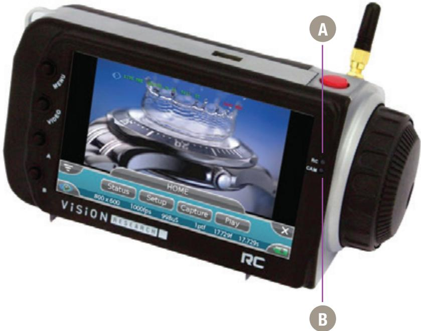
The RCU-2 LED indicators provide a visual representation of the camera's communication status, for the various operational states of the camera, see the table below.
