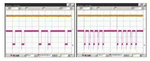
The image on the left shows a two-frame burst with the f-sync rate, (camera/sample rate), set to 500fps, the burst period set to 700 microseconds, and the exposure set at 200 microseconds. The image on the right shows a five-frame burst with the f-sync rate, (camera/frame rate) set to 200fps, the burst period set to 700 microseconds, and the exposure set at 200 microseconds.
